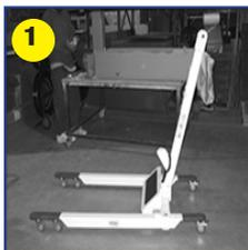
1. Remove all packing wrap from the lift base. Remove the two bolts, washer and nuts from the base. Insert lift mast into position securing with the 2 bolts supplied. Place washer and nut on the end of the bolt and tighten using a 3/4" wrench.
