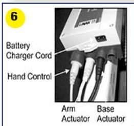
6. Looking at the bottom of the battery pack, starting at the left, plug in the hand control cord, next plug in the arm actuator cord and then base (black cord) actuator cord. The cord that plugs into the wall is used to charge the battery, plug it in above the other outlets as indicated. Actuator
