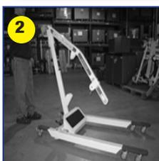
2. Remove the bolt at the top of the lift mast. Place the lift arm in place. Be sure when placing the bolt through to place the smaller washer on the outside of the mast, then the larger washers next to the arm. See picture below for proper placement. Secure nut with 9/16" wrench and #3 allen, then tighten
